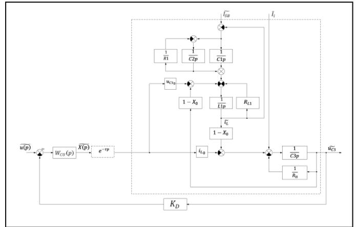
Fig. 3. The shunt converter’s linearized mathematical model with input filter and control system.
