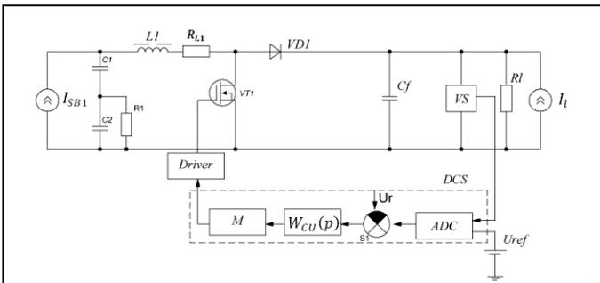
Fig. 1. The shunt converter’s scheme with digital control system.
