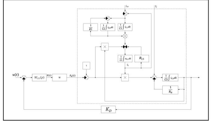
Fig. 2. The shunt converter’s mathematical model with input filter and control system.
