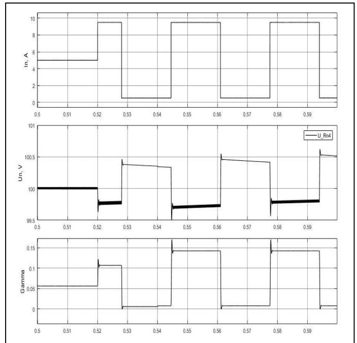
Fig. 8. Diagrams load voltage ( $U_n$ ), the control signal at the SB channel PWM modulator ( $\Gamma_{BS}$ ) input and load resistance ( $R_n$ )
