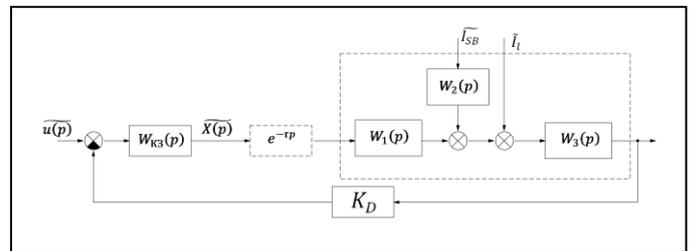
Fig. 4. The shunt converter’s simplified linearized mathematical model with input filter and control system
