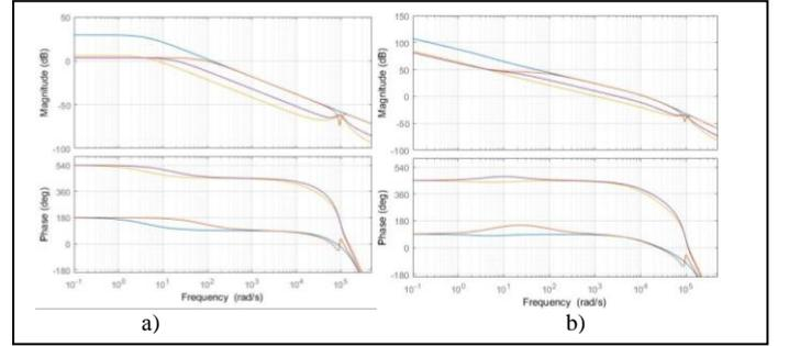
Fig. 6. Frequency characteristics: a) open uncorrected system, b) open corrected system.
