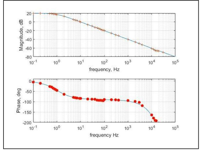
Fig. 5. LAFR and LPFR of the simulation ('+') and mathematical (blue line) models.
